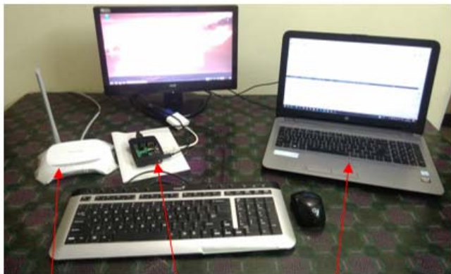
Access point Raspberry pi MQTT Broker 192.168.0.103 Client Python Scripts 192.168.0.104
