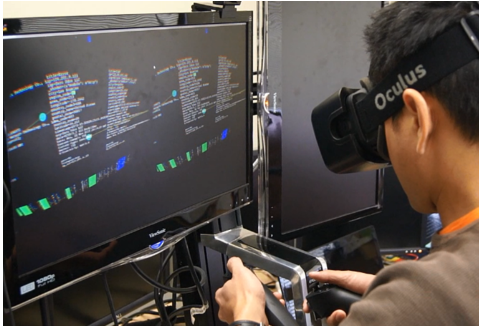
Figure 1: An immersive, head mounted display visualization for viewing text records from the Shodan database of Internet connected devices. The user is provided with a two handed interface for navigating and manipulating text.
