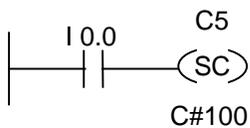
The counter C5 is preset with the value of 100 if there is a positive edge at input I0.0 (change from "0" to "1"). If there is no positive edge, the value of counter C5 remains unchanged.
