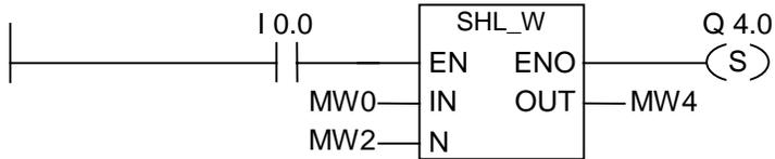
The SHL\_W box is activated by logic "1" at I0.0. MW0 is loaded and shifted left by the number of bits specified with MW2. The result is written to MW4. Q4.0 is set.
