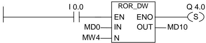
The ROR\_DW box is activated by logic "1" at I0.0. MD0 is loaded and rotated to the right by the number of bits specified with MW4. The result is written to MD10. Q4.0 is set.
