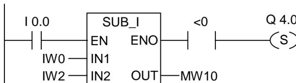
The box is activated by signal state "1" at I0.0. If the value of IW0 is lower than the value of IW2, the result of the math function "IW0 - IW2" is less than "0". Q4.0 is set if the function is properly executed and the result is **less** than "0".
