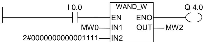
The instruction is executed if I0.0 is "1". Only bits 0 to 3 of MW0 are relevant, the rest of MW0 is masked by the IN2 word bit pattern:
