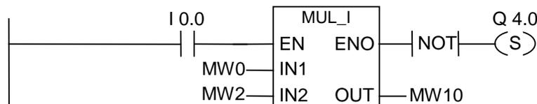
The MUL\_I box is activated if I0.0 = "1". The result of the multiplication MW0 x MW2 is output to MD10. If the result was outside the permissible range for an integer, the output Q4.0 is set.
