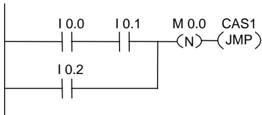
The edge memory bit M0.0 saves the old RLO state. When there is a signal change at the RLO from "1" to "0", the program jumps to label CAS1.
