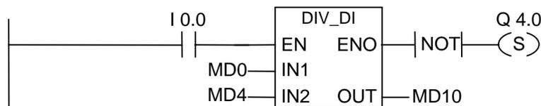
The DIV\_DI box is activated if I0.0 = "1". The result of the division MD0 : MD4 is output to MD10. If the result was outside the permissible range for a double integer, the output Q4.0 is set.
