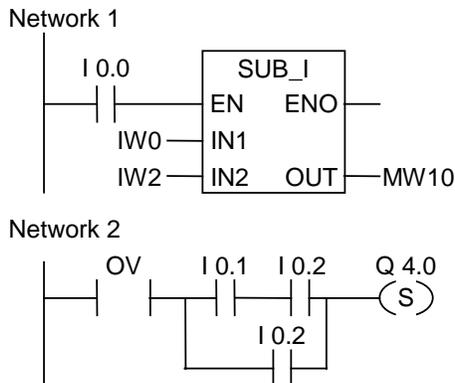
The box is activated by signal state "1" at I0.0. If the result of the math function "IW0 - IW2" is outside the permissible range for an integer, the OV bit is set.
