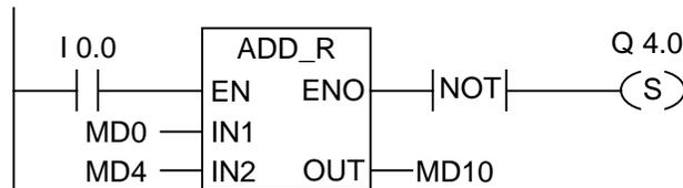
The ADD\_R box is activated by logic "1" at I0.0. The result of the addition MD0 + MD4 is output to MD10. If the result was outside the permissible range for a floating-point number or if the program statement was not processed (I0.0 = 0), the output Q4.0 is set.
