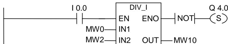
The DIV\_I box is activated if I0.0 = "1". The result of the division MW0 by MW2 is output to MW10. If the result was outside the permissible range for an integer, the output Q4.0 is set.
