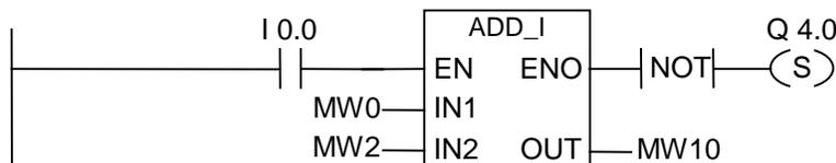
The ADD\_I box is activated if I0.0 = "1". The result of the addition MW0 + MW2 is output to MW10. If the result was outside the permissible range for an integer, the output Q4.0 is set.
