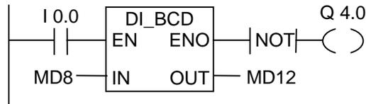
If I0.0 is "1", then the content of MD8 is read as a double integer and converted to a seven-digit BCD number. The result is stored in MD12. The output Q4.0 is "1" if an overflow occurred, or the instruction was not executed (I0.0 = 0).
