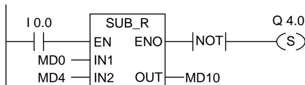
The SUB\_R box is activated by logic "1" at I0.0. The result of the subtraction MD0 - MD4 is output to MD10. If the result was outside the permissible range for a floating-point number or if the program statement was not processed, the output Q4.0 is set.
