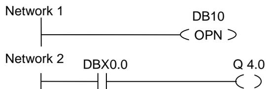
Data block 10 (DB10) is opened. The contact address (DBX0.0) refers to bit zero of data byte zero of the current data record contained in DB10. The signal state of this bit is assigned to the output Q4.0.
