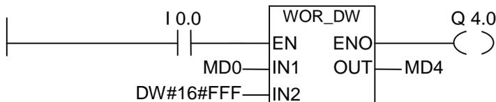
The instruction is executed if I0.0 is "1". Bits 0 to 11 are set to "1", the remaining MD0 bits are not changed:
