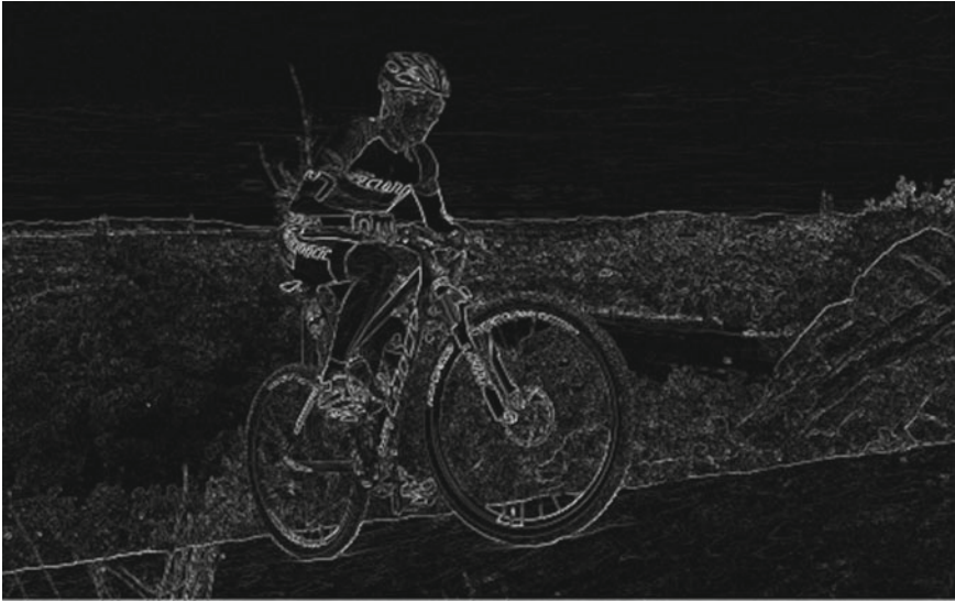
Fig. 8.3 The calculated energy function of the cyclist image
